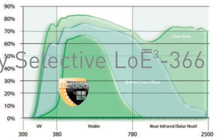
The special coating distinguishes desirable visible light from unwelcome UV and near-infrared rays (NIR). The result is the ultimate in solar heat control, fading protection and visibility.
